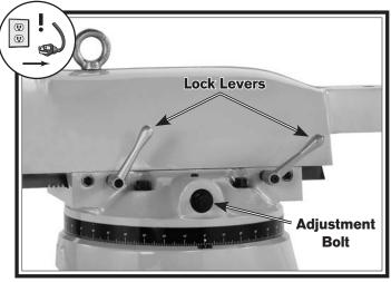
Figure 31. Ram back-and-forth movement controls.
